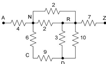
The resistance value is given next to each resistor. Connection points (wires connecting two or more resistors together, are denoted by an uppercase letter. A and Z are reserved for the names of the connection points which are the endpoints of the circuit. Our goal is to calculate the equivalent resistance of the circuit (i.e., the equivalent resistance between A and Z).
