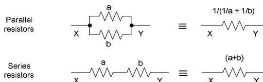
The equivalent resistance of a well-formed series-parallel resistor <sup>1</sup>circuit can be determined by successively replacing a series or parallel resistor pair by the single equivalent resistor, until only one is left. If this technique fails, the circuit is not well-formed.
